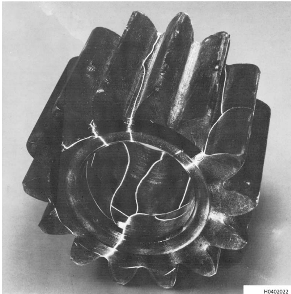
Figure 3-41. Typical Magnetic Particle Indications of Cracks
