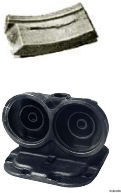
Figure 3-59. Magnetic Particle Indications of Defects in Castings
