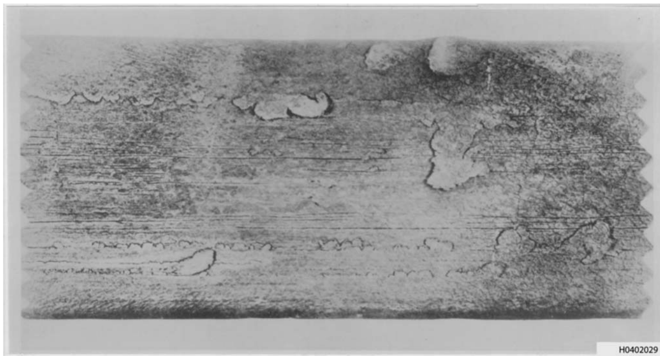
Figure 3-48. Scabs on the Surface of a Rolled Bloom
