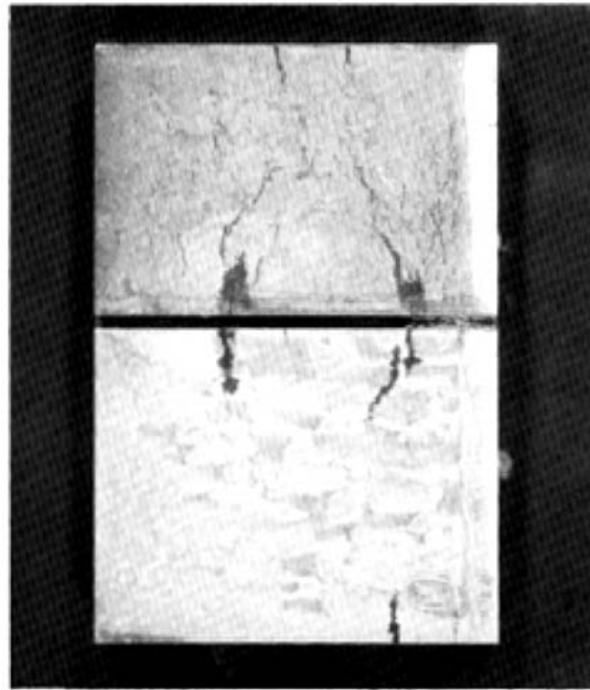
Figure 2-23. Cracked, Aluminum Panel Comparing Results of an Optimum Thickness Layer of Developer (Top) to an Excessive Thickness Layer of Developer (Bottom)
