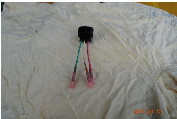
This is the new plug sourced from a Chinese company, to join to the new Sensor which makes it weather proof, more professional and cost about 12 cents + post, ever tried to get, 1 genuine plug for a late model loom?
