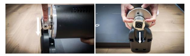
3. Gently push the tubular module down until the two small spring fasteners on the sides of the bracket click in.
