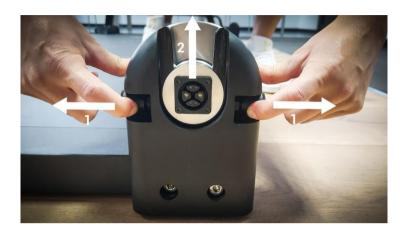
This action makes it possible to slide out the pin (normally engaged by the bracket) and then lift out the whole tube.
