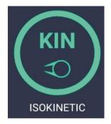
**KIN**: isokinetic load. In this mode you do not set a load (except for maximum load) but the movement speed imposed by the machine. The user will oppose resistance based on his/her strength.
