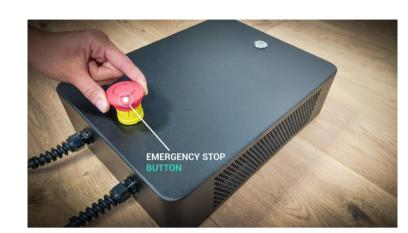
3) Check that the red emergency button has not been activated. If active, turn it clockwise.
