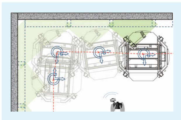
Figure 3. Route planning and execution by a human operator.
