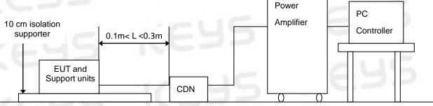
For the actual test configuration, please refer to the related item – Photographs of the Test Configuration Note: 1) The EUT is setup 0.1 m above Ground Reference Plane
