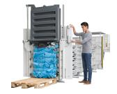
Safeguarding of the operating area with infrared light curtains for maximum operator safety
