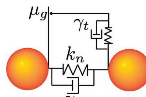
Linear springs with friction & dissipation
