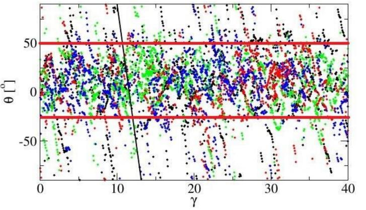
Interaction with neigbors leads to an orientation distribution with the average alignment <u>NOT</u> parallel to the main flow.
