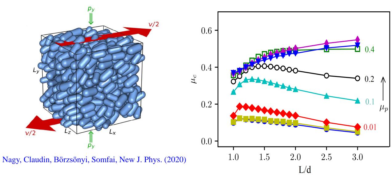
In laboratory experiments with effective friction as a function of grain elongation. We find the largest shear force for slightly
