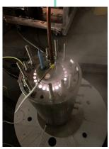
Designed to operate at 500 ATM, 600°C, 500kW
