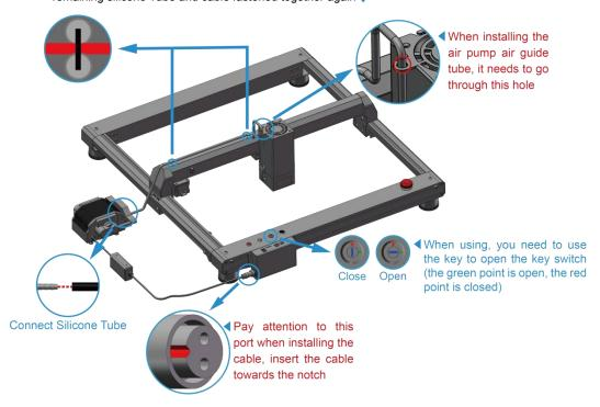
Tip: After the motor cables are connected, please manually move the X or Y axes slowly and DO NOT manually move the axes quickly, otherwise it will cause damage to the motherboard
