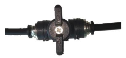
c) Turn the valve switch clockwise 90° to open the valve (as shown below)
