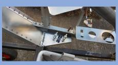
**2** Both toggles fitted to the bracket – right-hand side cockpit.
