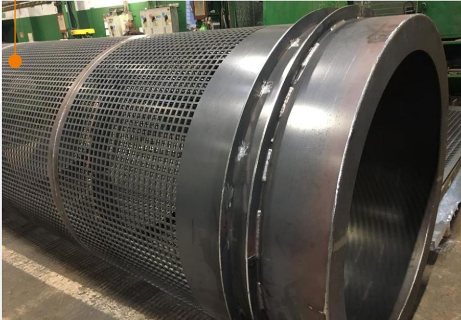
● Drum sieves with replaceable mesh
