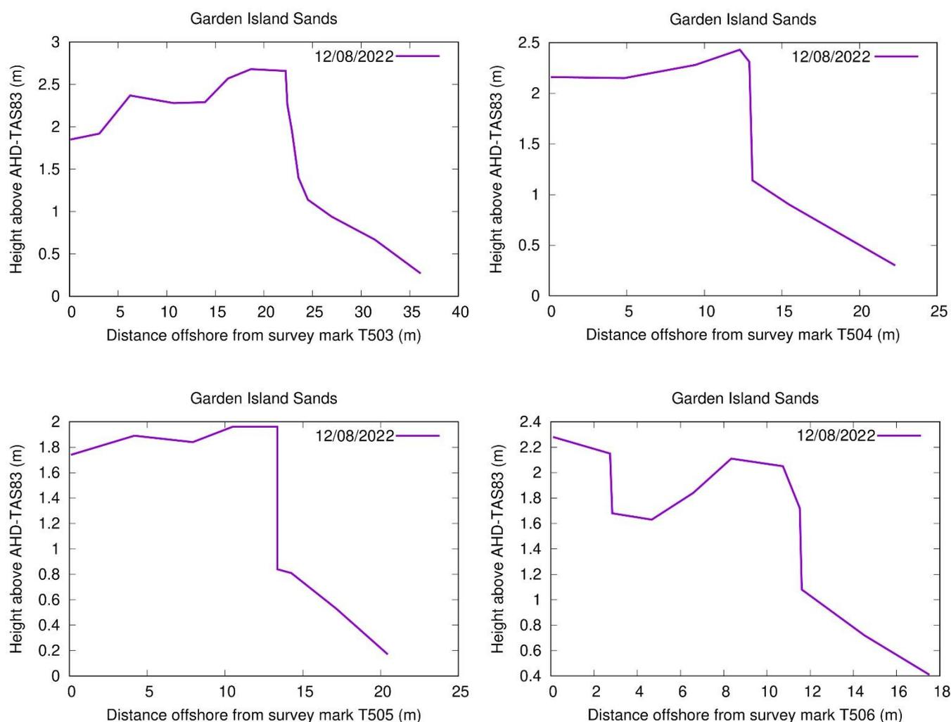
**Figure 17: The first TASMARC profiles surveyed from the 4 survey markers at Garden Island Sands Beach, on 12<sup>th</sup> August 2022.** Survey plots prepared by Nick Bowden; scales are in metres. Note that the vertical scale is exaggerated compared to the horizontal scale, which makes all landform features appear steeper and higher than they really are (albeit the vertical erosion faces are indeed as steep as they appear, but their height relative to the horizontal scale is exaggerated).
