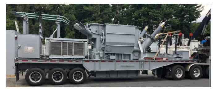
HIGH VOLTAGE: 69000 X 138000 DELTA LOW VOLTAGE: 13200Y/7620 X 26400Y/15240 TAPS: 144900-141450-138000-134500-131100 TAPS: 72450-70725-69000-67275-65550
