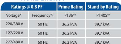
The above ratings represent the generating set capability guaranteed within  $\pm 3\%$ at the reference conditions equivalent to those specified in ISO 8528/1 standard.
