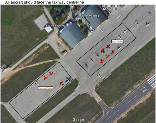
Last flight of the day, always use at least one (1) tie down. If strong winds are forecast, or aircraft will not be used again anytime soon, aircraft must be secured at 3 points using the tie downs in the cabin. Aircraft must be covered, if cover is available.
