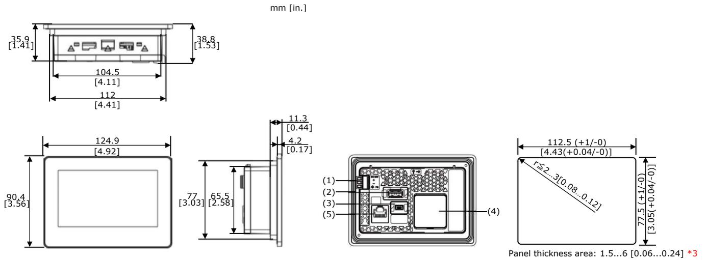
(1) Power Connector (2) USB (Type A) Interface (3) USB (mini-B) Interface (4) RTC Battery Set Cover (5) Ethernet Interface mm [in.]
