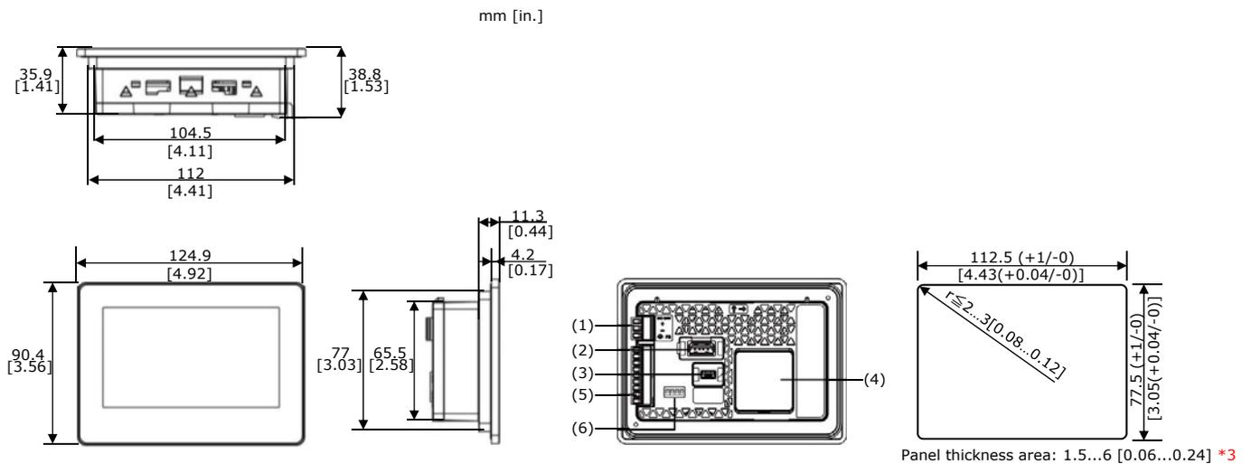
(1) Power Connector (2) USB (Type A) Interface (3) USB (mini-B) Interface (4) RTC Battery Set Cover (5) Serial Interface (6) DIP Switch mm [in.]
