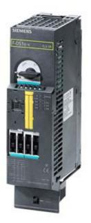
F-DS1E-X FOR ET 200S FAILSAFE DIRECT STARTER SETTING RANGE 0.3...3A MECHANICAL SWITCHING ELECTRONIC PROTECTION AC-3, TO 1.1KW/400V, CAN BE EXPANDED FOR BRAKE CONTROL MODULE FOR 2DI CONTROL MODULE
