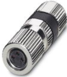
Sensor/actuator connector, female, straight, 3-pos., M8, Piercecon®, metal knurl, cable diameter max. 5 mm
