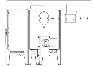
Align the Heat Shield on the slots to cover the gap between the Twin Wall and the Top Plate. The overlap must be at least 10mm.
