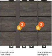
Side adaptor with T trim profile Butt join applications
