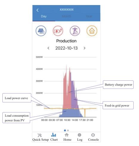
The above combination day chart shows the PV production power distributed with three parts:
