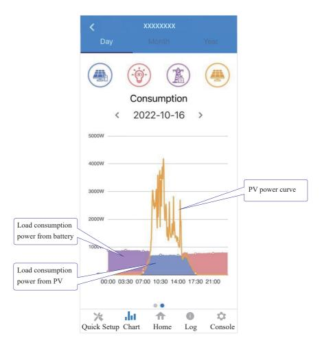
The above combination day chart shows the load consumption power from three parts:
