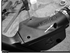
**15.** Tighten all the screws using a philips screwdriver.
