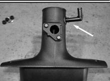
**22.** Install the provided grommet to the hole on intake plenum. Install the 90 degree plastic elbow long side first to the grommet and secure.
