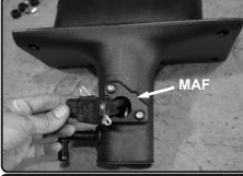
23. Remove the MAF sensor from the stock air box, install the MAF sensor into the new intake plenum.
