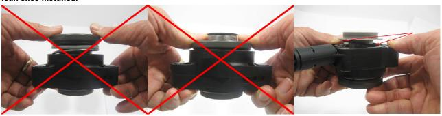
Never spray brake cleaner or solvents in or around the CSC. This can cause the seals to swell and wash away the assembly lubricant.
