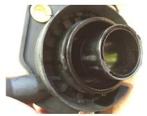
Off Axis Wear On Guide Tube
