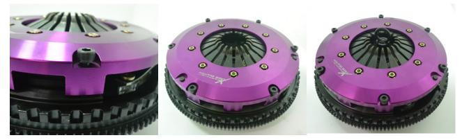
11. When the six M8 bolts have pulled the pressure plate up to the flywheel, torque all 6 bolts to 26 ft. Lbs/ 35 N.m.
