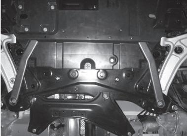
\*Periodically inspect and retorque all nuts and bolts after vehicle operation.
