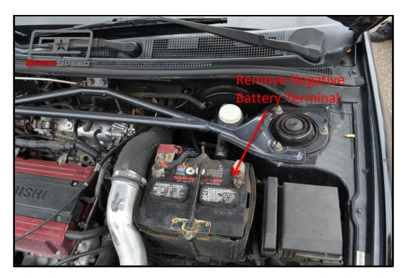
2. Next, remove your factory strut tower bar. This will be three (3) 14mm nuts on each side plus two (2) 14mm bolts in the center. Set it aside when you're done.
