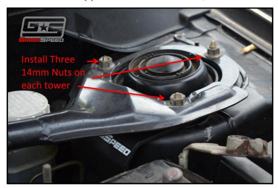
8. Now you're ready to install the stud, nuts and red cap. See the figure below to identify where each piece goes, noting that the allen key will fit into the end nearest the battery. Get this in there loosely at first.
