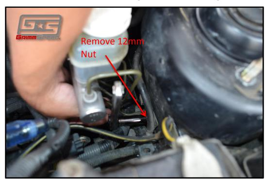
4. Now, remove the bolt that's grounding your battery cable to the strut tower. You'll need to flip it 180 degrees and bolt it back down to make room for the brace.
