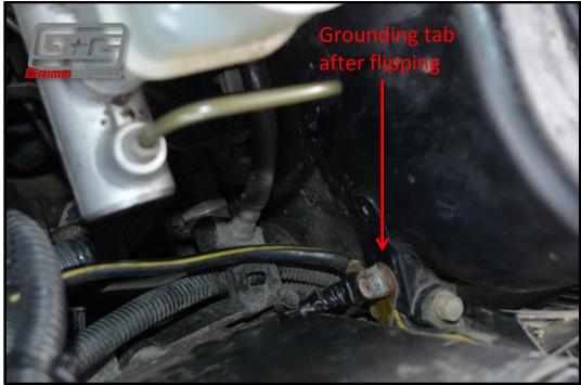
5. Now, there should be plenty of room to slip the brace down so that the tab on the bottom straddles the stud and the three studs at the top of the strut tower sit nicely in the brace. Reinstall the 12mm nut towards the bottom of the brace.
