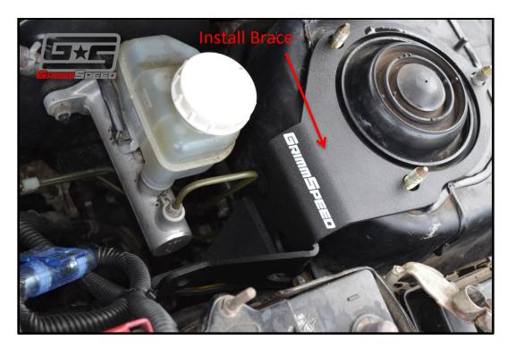
6. Now set your strut tower bar back in place. Before moving forward, you'll want to reinstall the two 14mm bolts attaching it to the firewall. If you're having any trouble an extra set of hands to push down on the brace a bit can make the job much easier.
