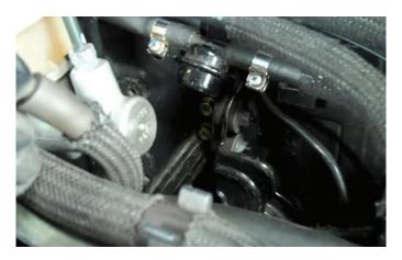
6. Move master cylinder brace into place. It slips underneath the fuel lines.
