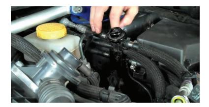
12. On some STI models, the plastic clip will not be reused as the fuel rail pulse dampers are larger. Loosen fuel lines and rotate to get in a position where they can be zip tied to the black metal bracket. Ensure the hoses, lines, and dampers are not
