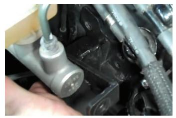
8. Take the bracket from step 5 and install it above the master cylinder brace lining up the 2 holes.
