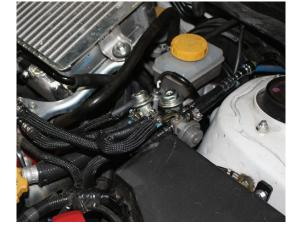
13. Assemble stud, nuts and pressure cup as shown in the picture. Do not tighten the nuts.
