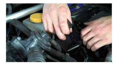
7. Install one of the 3 shorter M6 bolts into the top left hole of the master cylinder brace and thread it in by hand. Using the remaining short M6 bolts, thread into the 2 hole that are below the first bolt that was installed.
