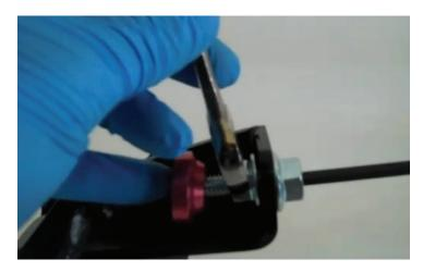
15. Now tighten the other nut to lock the adjustment into place.
