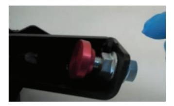
14. Using a 15mm wrench and 5mm hex key, insert hex key into stud and tighten the nut closest to the master cylinder which will extend the stud. Ensure that the other nut is loose. When the pressure cup makes contact with the master cylinder, tighen the nut an additional 1/2 to 1 turn.
