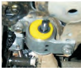
View of right hand side of vehicle showing correct maximum positive caster position
