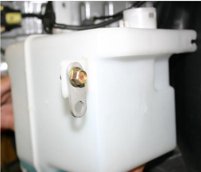
Washer Bottle Shown with Flat Bracket Installed
