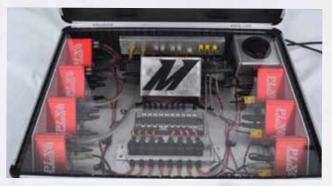
Figure 1: PLX sensor modules were used to monitor engine pyrometers.
