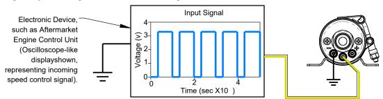
Refer to above Example 5, for use with the Fuelab Electronic Fuel Pressure Regulator, Models 52901 and 52902, that creates its own pulsed signal. These regulators automatically control the fuel pump, without the use of switching means or other components such as described in examples 2 and 3. Refer to instructions for the Electronic Regulator for proper wiring and installation.
