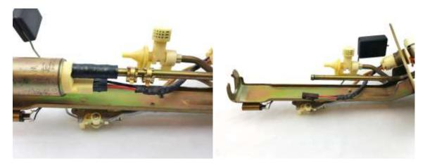
2 – prep the DW300 by installing the fuel sock and retainer. Start installation of the retainer by pressing it on with your thumb, then use a 4-5mm deep socket to press it on the rest of the way
