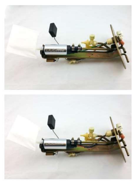
4 – reinstall the assembly into the fuel tank and attach a length of hose to the outlet of the pump assembly allowing it to drain into a fuel safe container and prime the fuel pump assembly
