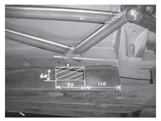
6.) The undercover tray will need to be modified (cut). Cut the shaded area to give clearance to the newly installed bar. (Photo shows passenger side, do the same for the other side)
