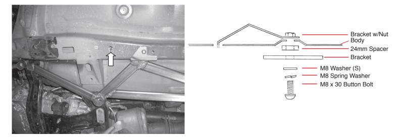
5.) Slide in the included Bracket/Nut and align to the hole shown above. Install by using the M8 x 30 Button Bolt, M8 Spring Washer, and M8 Washer (S) like the diagram above.
