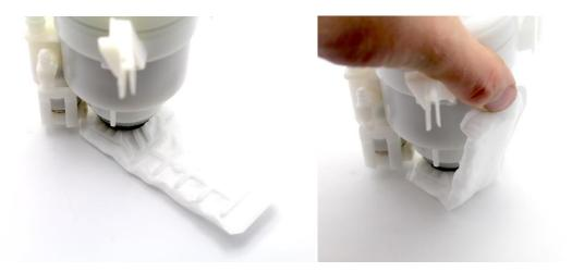
10 - reinstall the top assembly, plug in electrical connector to the top assembly, and install c-clip
