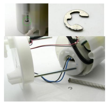
2 – pull out top assembly, take note of the routing of the black fuel lines
