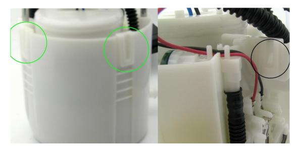
4 – lift and remove the center from the bucket.
