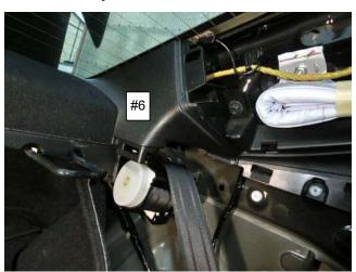
7 Remove Seat Belt Retractor Assy. (Remove x2 Bolts)
