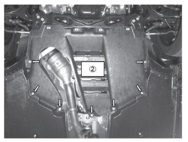
2.) Remove the rest of the undertray by taking off the bolts indicated with the arrows.
