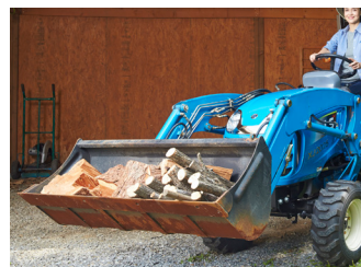
High Capacity Front Loader Features 1,276 Lbs. Of Lift Capacity At Pivot Pins
