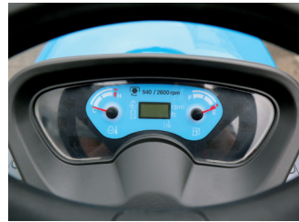
Illuminated Dash With Digital RPM Provides Excellent Operator Visibility
