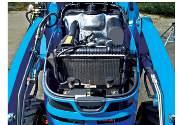
Engine Compartment Access Excellent Access For Preventative Maintenance
