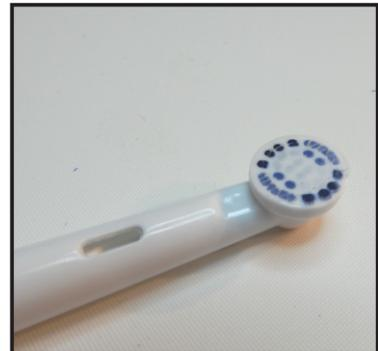
Then, punch a piece of smooth plastic from Styrene, or other flat hard plastic (such as a plastic grocery tray) with a 5/8" round punch. Glue the plastic onto the brush head, with a good plastic glue, and clamp until dry.
