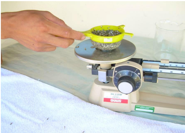
Figure 4-1: Estimating fry numbers by gravimetric and water displacement method (Source: Meyer & Meyer, 2007)
