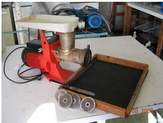
Plate 8-3: Different size pellets are made by extruding the mash (mixture of ingredients) through dies with different size holes and then cutting the strands to the required length (Gonzalez & Allan, 2007)
