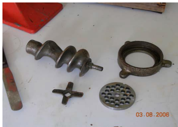
Plate 8-3: Different size pellets are made by extruding the mash (mixture of ingredients) through dies with different size holes and then cutting the strands to the required length (Gonzalez & Allan, 2007)
