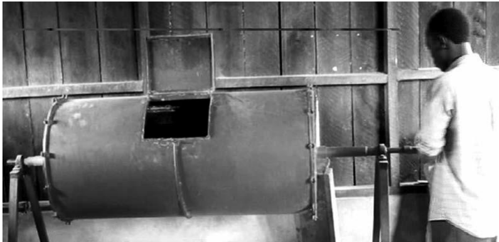
Plate 8-2: A hand-operated mixer is used to mix feed ingredients at Sagana Aquaculture Centre.
