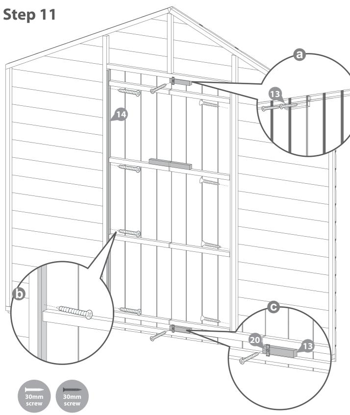
a First line up the door blocks at the top and bottom of the doors. Then fix with 2x30mm screws by screwing through the outside of the door into the block.
