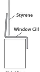
Place the plastic window cill onto the Window Panel and silicone in place as shown on both diagrams to the left.
