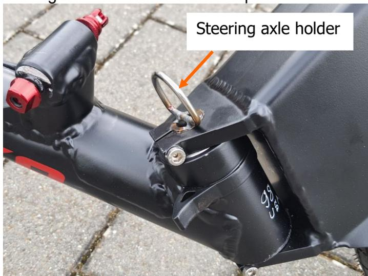
Push the steering axle completely in the hole. Note: it helps when turn the axle while pushing.
