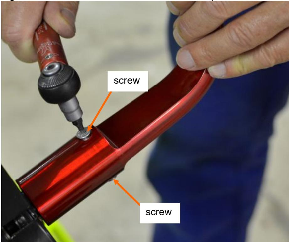
**Security check:** All screws of the arm cranks must be completely inside the arm cranks.
