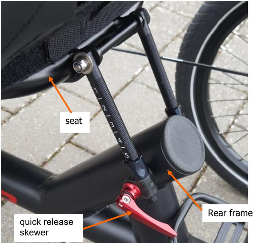
Tighten the quick release skewer
