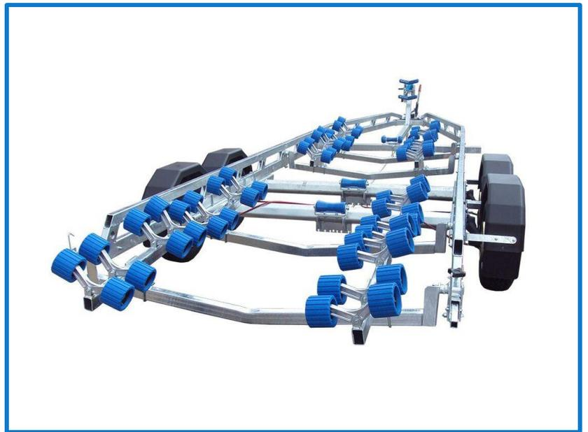
Everything on this trailer is adjustable, so it can fit most hull shapes.
