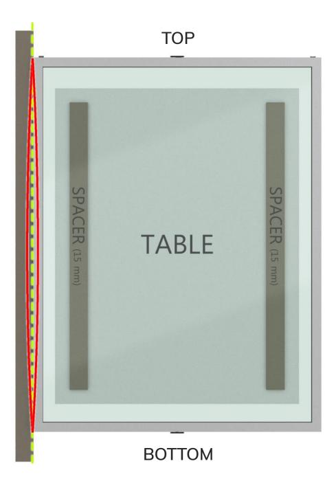
Make sure the starting profile is 100% straight! If not, use a rubber hammer to straighten profile.
