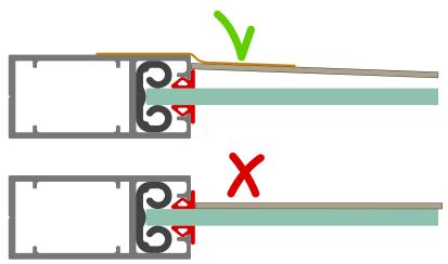
Use masking tape to keep the guide in place, on top of the rubber!.
