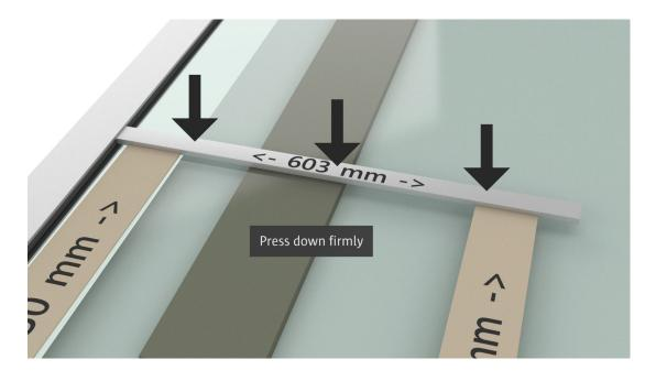
Place one end of the grid profile in the rubber gap, use the length guides to position it onto the glass and press down firmly.
