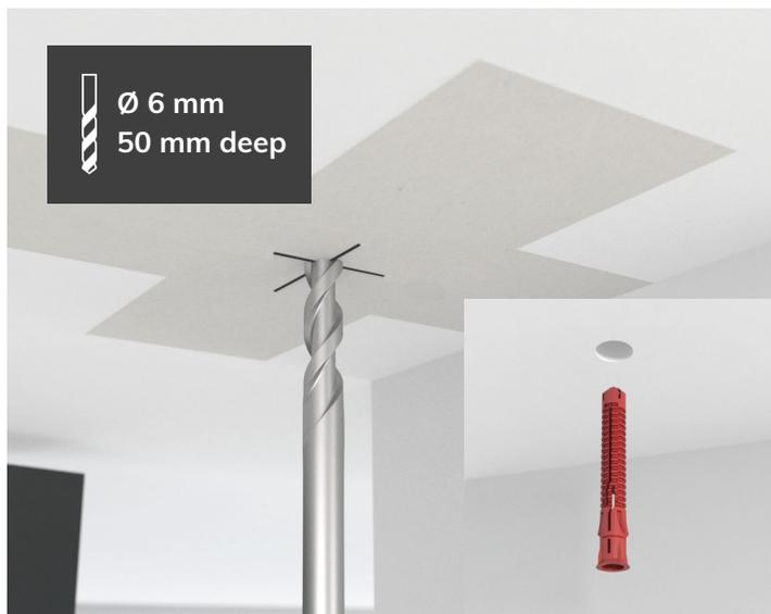
Drill the hole and install the magnet with Hilti plug and screw.
