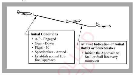
**Note:** If during the ILS final approach exercises the decision is made to go-around, the Approach to Stall or Stall Recovery maneuver must be completed before the go-around is initiated.
