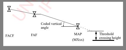
**Note:** The final approach course fix (FACF) is typically located on the final approach course approximately 7 NM before the FAF. The FAF referred to in the following procedures refers to the charted FAF and is intended to mean the point at which the final approach descent is begun.
