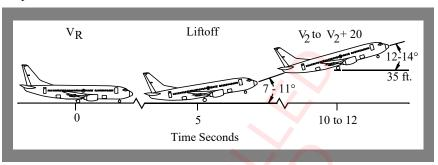
Retract the landing gear after a positive rate of climb is indicated on the altimeter. Retract flaps in accordance with the technique described in this chapter.
