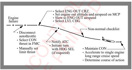
**Note:** If the airplane is at or below maximum ENG OUT altitude when an engine becomes inoperative, select the MOD ENG OUT CRZ (ENG OUT CRZ for FMC U10.3 and later). Maintain engine out cruise speed using manual thrust adjustments.
