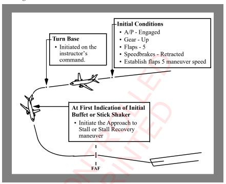
**Note:** The instructor commands initiation of the turn to base when the airspeed is at minimum maneuver speed (top of the amber band), or at flap 5 maneuver speed for airplanes without an amber band display. This ensures the initial buffet or stick shaker occurs during the turn.
