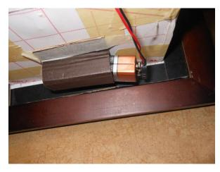
Hook up the battery, and place in the battery cover. Tape all electrical wiring firmly to the outside of the box.
