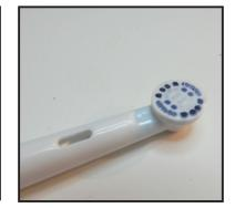
Then, punch a piece of smooth plastic from Styrene, or other flat hard plastic (such as a plastic grocery tray) with a 5/8" round punch. Glue the plastic onto the brush head, with a good plastic glue, and clamp until dry.
