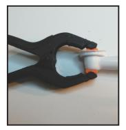
Just punch out 5/8" circles of your chosen sandpaper, peel the backing off, and apply to your new sanding toothbrush. When the grit wears out, just peel off the worn out sandpaper and apply another piece.
