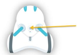
To turn your Photon on, press and hold the switch on button placed on the robot's head for 2 seconds. Robot's antenae and eyes will start blinking.
