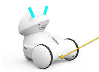
Charging plug is located in the rear. When Photon is being charged, its antennae are blinking using red colour. When battery is full Photon' antennae' colour changes to green. When this happens, you can unplug your robot and start playing.
