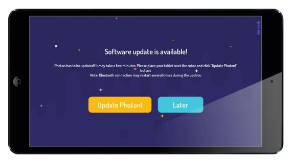
Do not turn your robot and mobile device off while the update is in progress. After clicking the "Update Photon!" button new software will be installed. While updating, Photon's antennae and eyes will be blinking irregularly. After a couple of minutes Photon will make a turning off noise and turn on again. When the update is finished, a communicate will appear on the screen.
