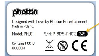
Each robot has its own ID number that helps to identify robots in the app. ID numer consists of 3 digits and it is placed on Photons bottom part.
